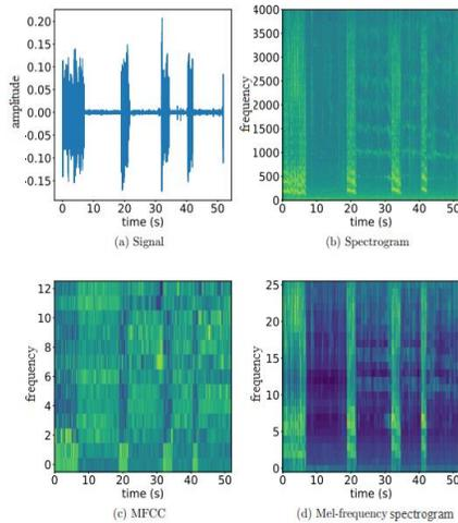
**Fig. 3.** Conversion of raw audio signal into mel-frequency spectrogram for
