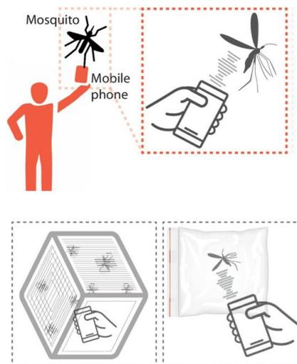
**Fig. 2.** Graphical illustration of mosquito sound collection in labs and open areas using mobile phones. Noise level  $\leq 50$  dB, distance between mobile microphone and mosquito  $\leq 50$  mm. A similar setup was used for dataset collection in [11].
