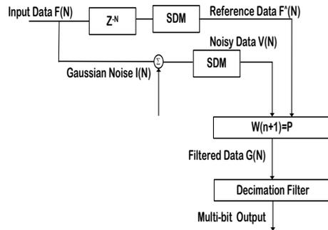
**Fig. 4:** Detailed Diagram of Proposed SDM-Based Corellationless Steepest-Descent Algorithm for Noise Removal.
