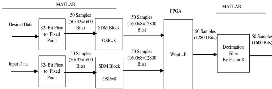
**Fig. 13:** MATLAB and FPGA Based Data Flow Diagram of Proposed Architecture.
