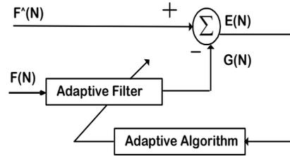
Fig. 2: The Block Diagram of Covnectional Adaptive Noise Canceller.
