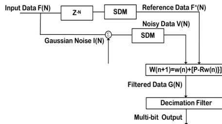
Fig. 3: Detailed Diagram of Conventional SDM- Based Steepest-Descent Algorithm for Noise Removal.
