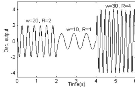
Fig 1: Change in frequency and amplitude of the oscillator (Source: [6])
