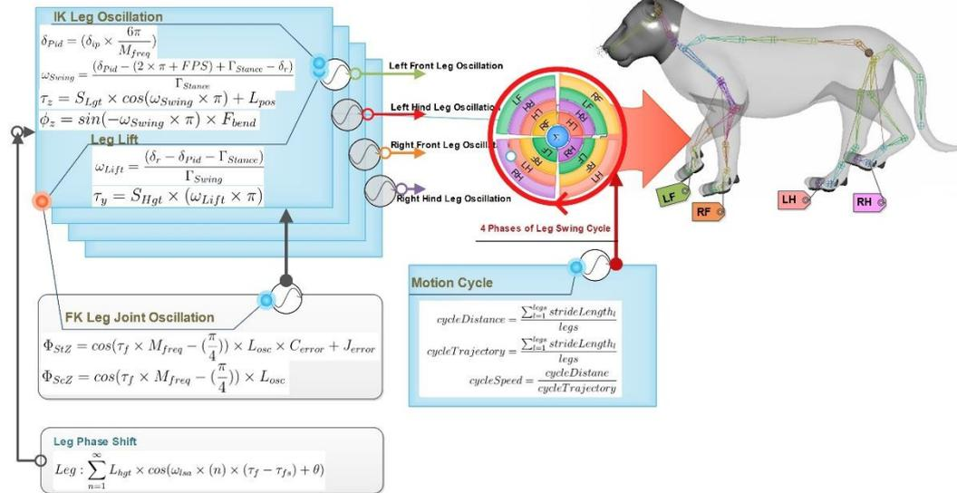
Fig 5: Mathematical model for CPG based Leg Simulation
