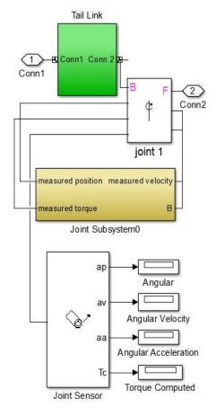
Fig. 4: Link joint subsystem of 10-link snake robot
