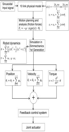
Fig. 1: System Block Diagram of a 10-link Snake Robot
