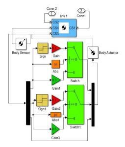
Fig. 7: Coulomb's friction module of an individual link
