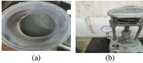
Fig. 2. (a) Powder Blending (b) Powder Compaction.
